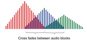
Figure F.7 Gain smoothing by the "overlap and add" process.
