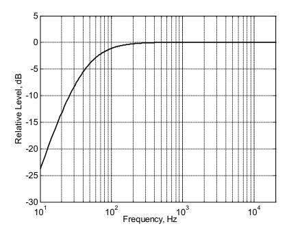
**Figure A.2** The RLB weighting curve.
