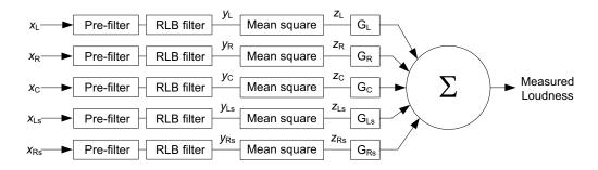
Figure A.1 Block diagram of multichannel loudness algorithm.
