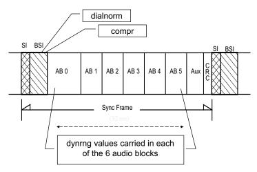
**Figure F.4** AC-3 DRC metadata placement in the bitstream.
