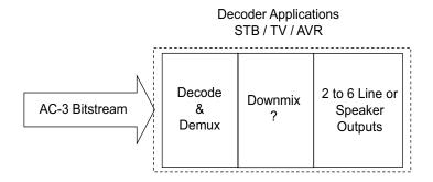
Figure F.2 AC-3 decoder requirements (Line Mode).
