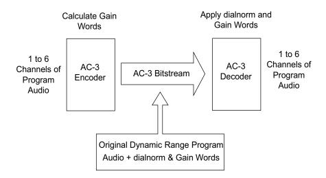
Figure F.1 AC-3 DRC basic concept.
