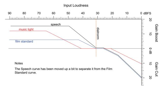
Figure F.9 DRC profiles input/output characteristics.
