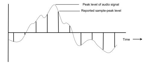
**Figure A.5** Continuous-signal peak level versus sample-peak.
