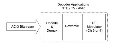
Figure F.3 AC-3 decoder requirements (RF Mode).
